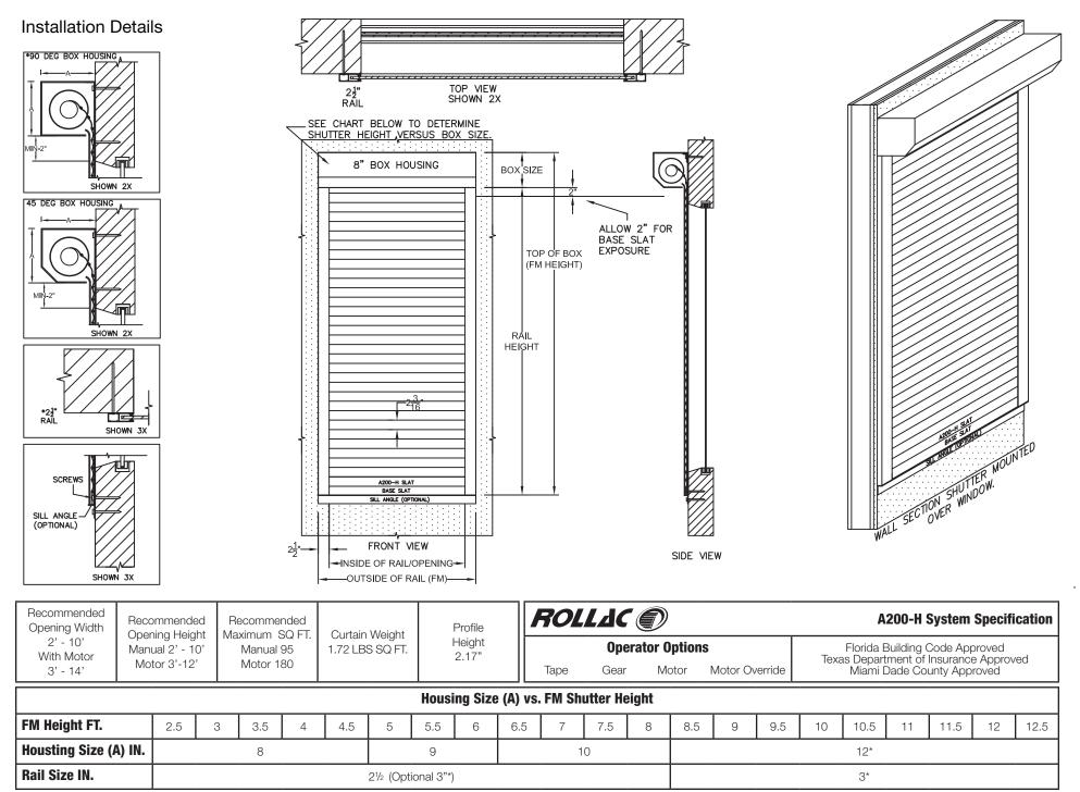
\*3" rail only available with 45 degree housing. 12" housing only available with 45 degree boxes. © 2015 Rollac
